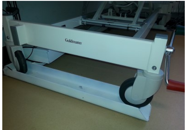
Figure 1. An image of the steel frame onto which the care bed (here a GB4 from Guldmann A/S) can be rolled on and off. Four load cell sensors are mounted underneath the steel frame.
